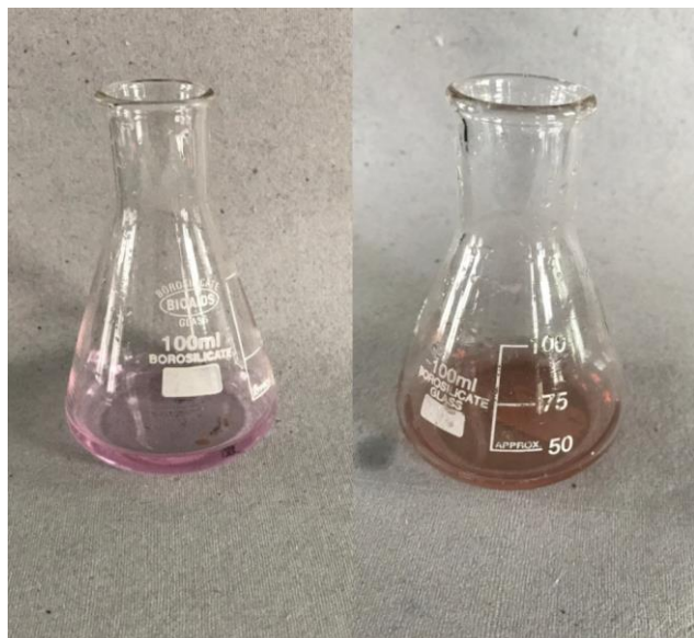
Fig.9. End point of acid-base titration using phenolphthalein and areca precipitate as indicator.
